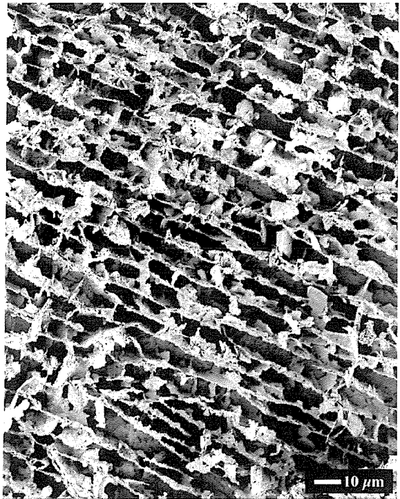
Fig. 5. Scanning electron microscopy showing clay card-house structure of mature fine tails at a void ratio of 5.
